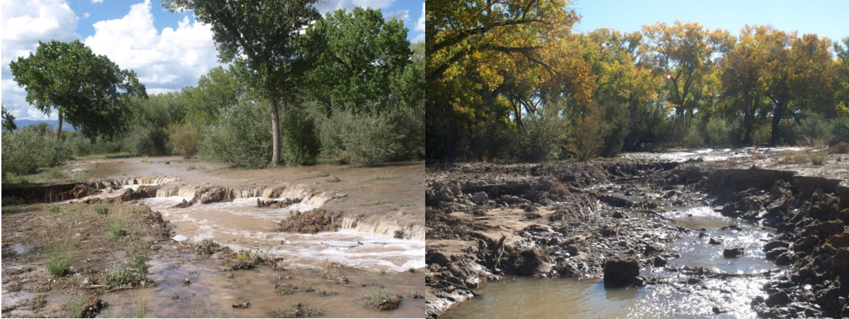
Figure 2 Incision on southern end of eastern terrace. Left: Vertical drop at one of the incision fingers during the overbanking flow. Right: One of the longer incision fingers. Photographs were taken on 9/17/2013 and 10/17/2013 respectively.
