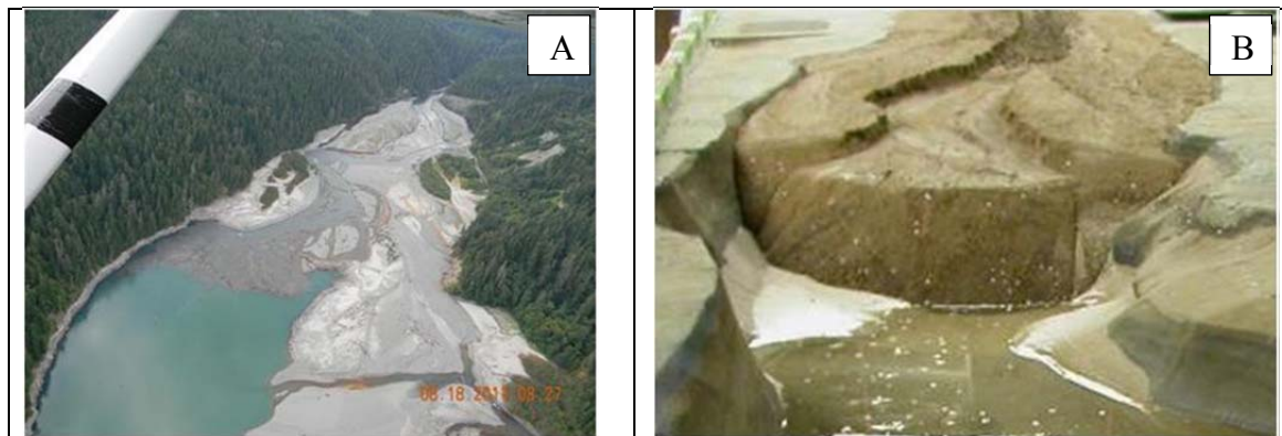
Figure 3. Photographs of sediment erosion and re-deposition at Lake Mills (A) as observed in August 2011 (16 feet of spillway drawdown prior to dam removal) and (B) in a laboratory model of Lake Mills conducted by Bromley (2007).
