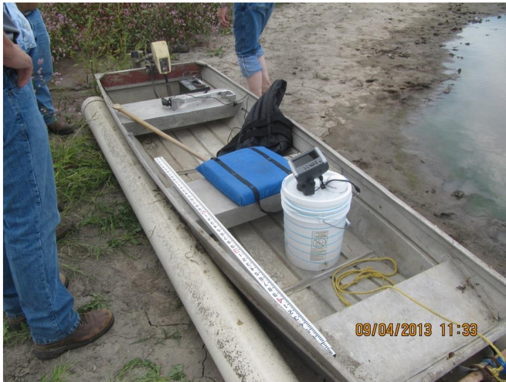
Figure 8 On-shore preparations. Transducer connected to transom mount (lying on its side on back seat of boat) with cable electrical running to depth finder mounted to bucket lid. Survey rod, used to confirm depth against finder reading, is shown at boat's starboard side.
