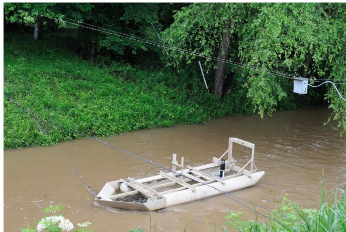
Figure 2. Deployment of the LISST on tethered floating platform in Goodwin Creek during 06/10/2014 runoff event.
