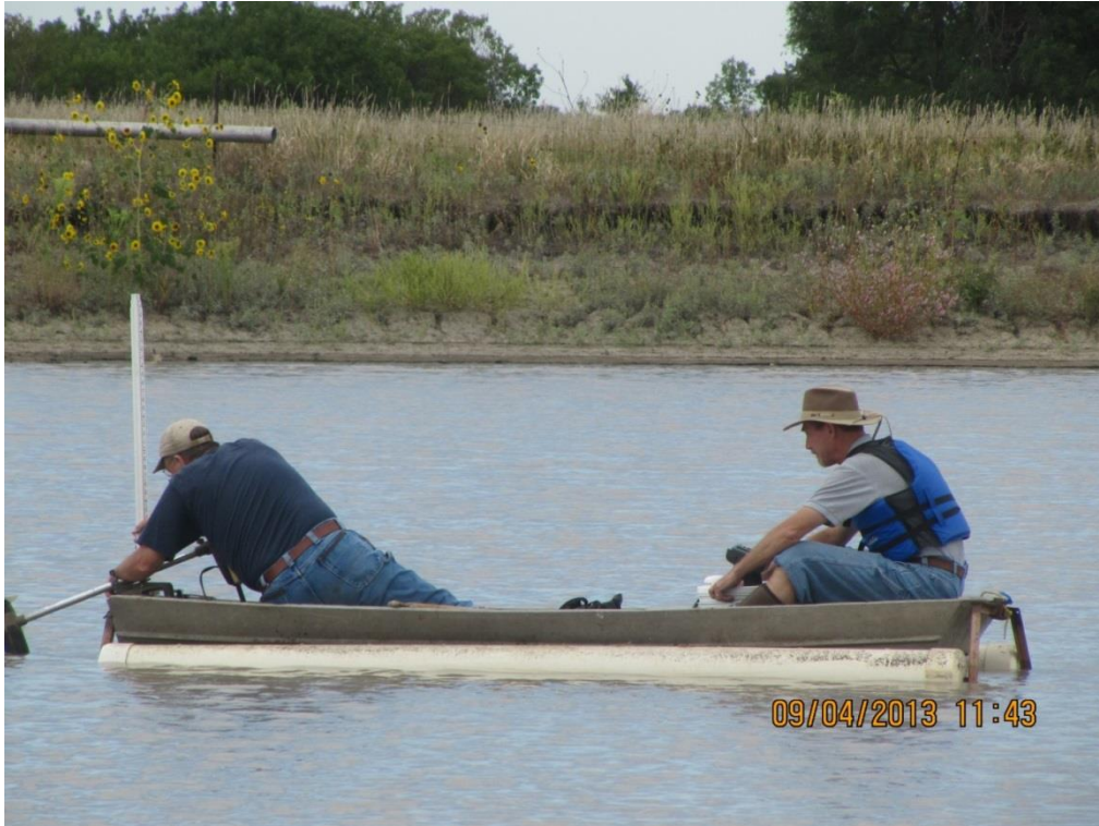
Figure 3 Manual depth readings are used to verify depth finder readings. This is done to confirm depth finder accuracy and/or determine the need for a correction factor.
