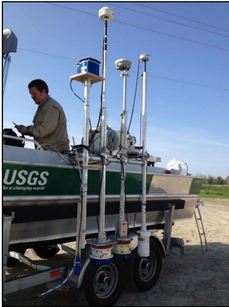
Figure 2 Mounting configuration for ADCPs used to measure apparent moving bed velocities in the Kootenai River at Crossport near Bonners Ferry, Idaho (USGS 12308500), May 17-18, 2012. ADCPs are (from left to right): TRDI StreamPro, TRDI 600 kHz Rio Grande, TRDI 1200 kHz Rio Grande, and SonTek/Xylem RiverSurveyor M9.
