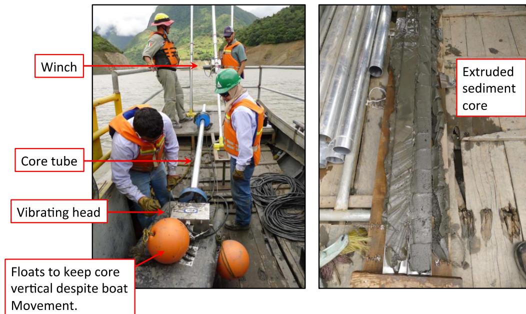
Figure 8 Battery operated vibracore used for sampling sand concentration near a hydropower intake.
