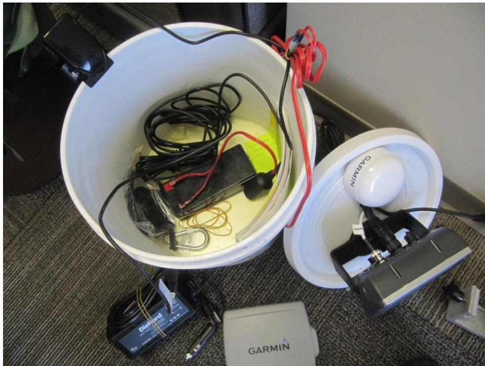
Figure 2 Depth finder system components: Garmin GSPmap 536s sounder/depth finder, dome antennae (both mounted on bucket lid), battery charger with vehicle adapter plug, 12V battery with vehicle adapter socket, and transducer clipped to bucket rim. Top of transom mount visible at lower right. The Garmin monitor cover shown removed at lower middle.
