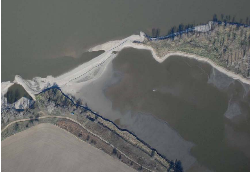
Figure 6 Typical Backwater at Low Winter Water Level Illustrating Entrance Sediment Bar
