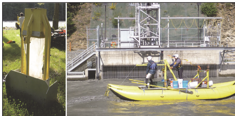
Figure 5 Photographs of the TR-2 (left) and the cataraft (right) used to measure bed load on the Elwha River
