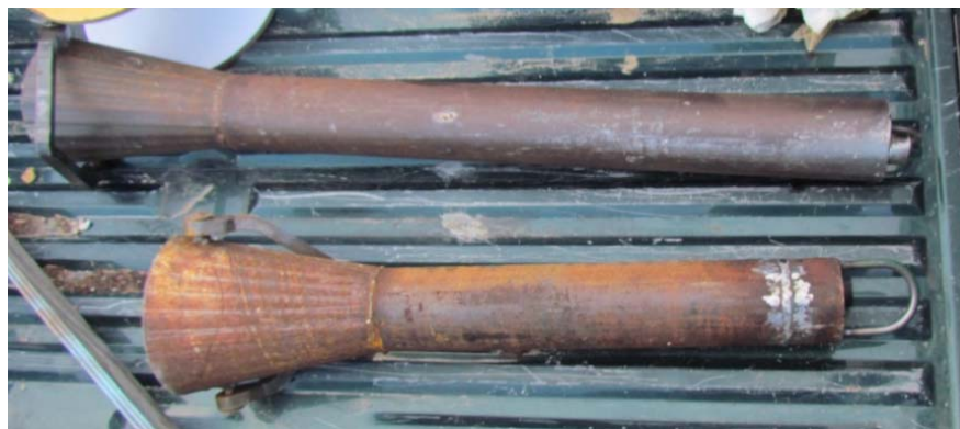
Figure 3 WES drag samplers: Original 4-ft long sampler (top); Sampler shortened by 11-inches (bottom).
