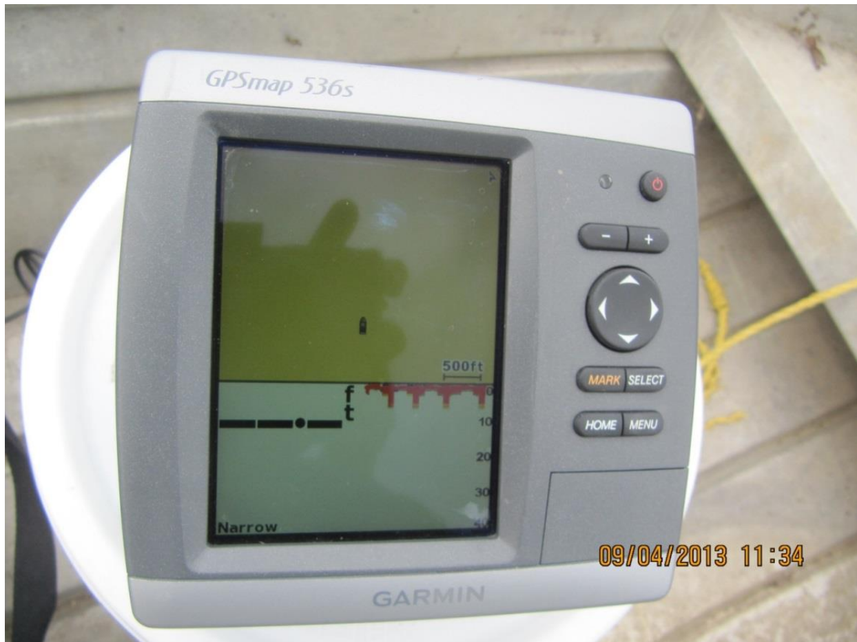
Figure 14 Dual display depth finder monitor readings of location, heading (top) and depth (bottom).
