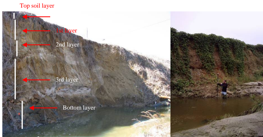
Figure 3. Representative streambank soil profiles observed along the modeling reach at Yonaba Creek in Blue Springs, MS
