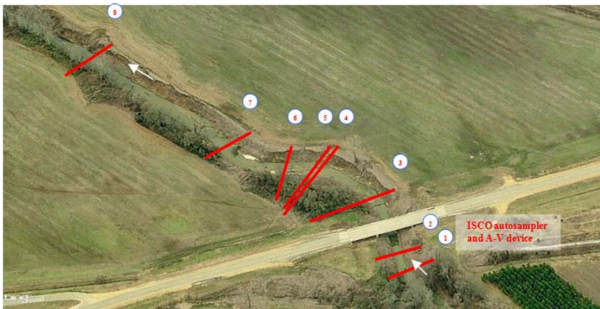
Figure 2. Yonaba Creek study site. Plan view showing the location of surveyed cross sections
