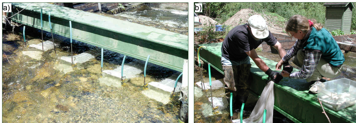
Figure 2: Bedload traps installed at E. St. Louis Cr. (a); Retying the net after emptying the contents into buckets (b).
