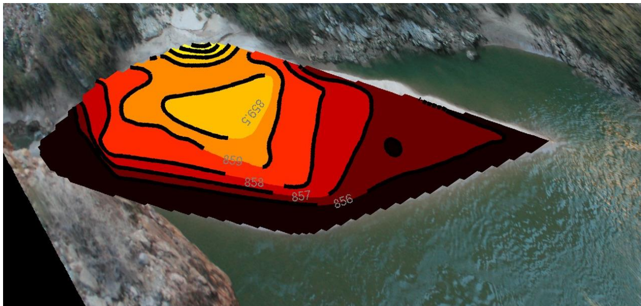
Figure 6 A colored DEM with contours of the RM 30.7 sandbar, overlain onto an orthorectified image of the bar after the 2012 controlled flood. This DEM was computed from the sequence of images taken during the flood shown in Figure 4, and associated stage elevations, following the methods summarized in Figure 4.
