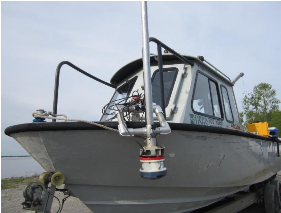
Figure 3 Boat Rim Mounted ADCP
