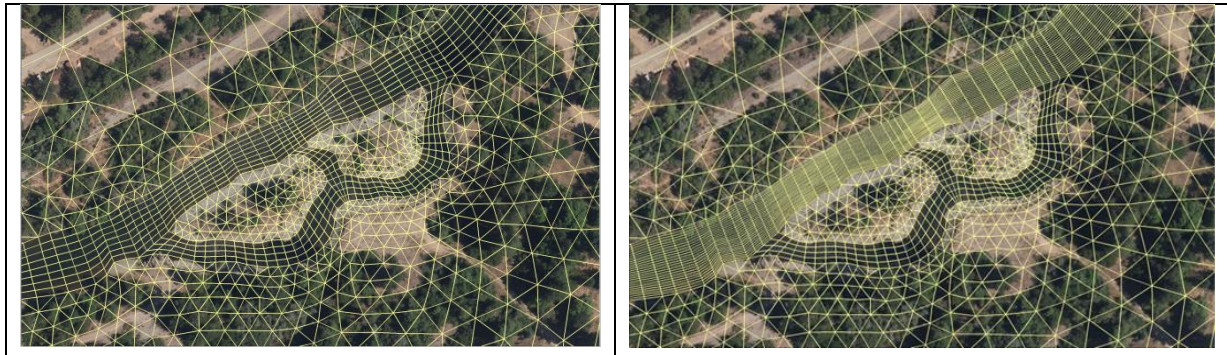
Figure 1 Comparison of the calibration mesh (left) and the habitat mesh (right)
