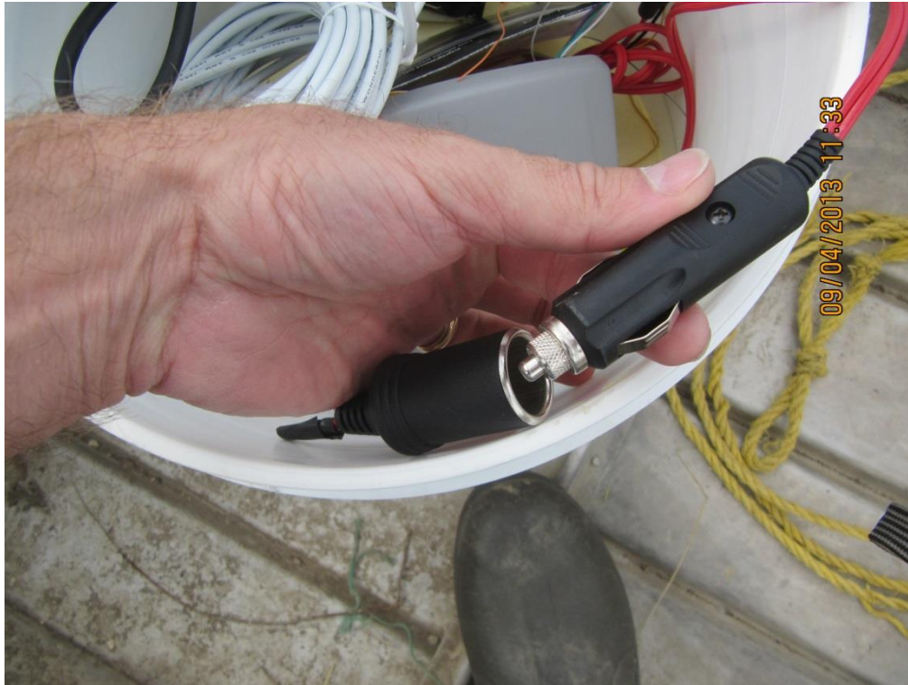
Figure 13 Power cable connection from depth finder plug (right) to 12V battery socket (middle).
