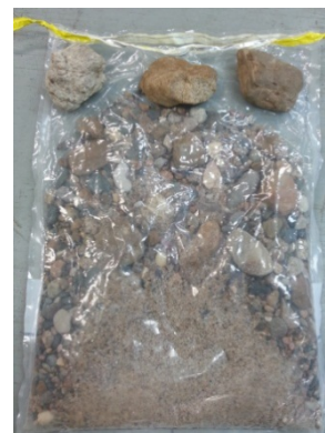
Figure 5c Poorly sorted sample, 3 D_{max}
