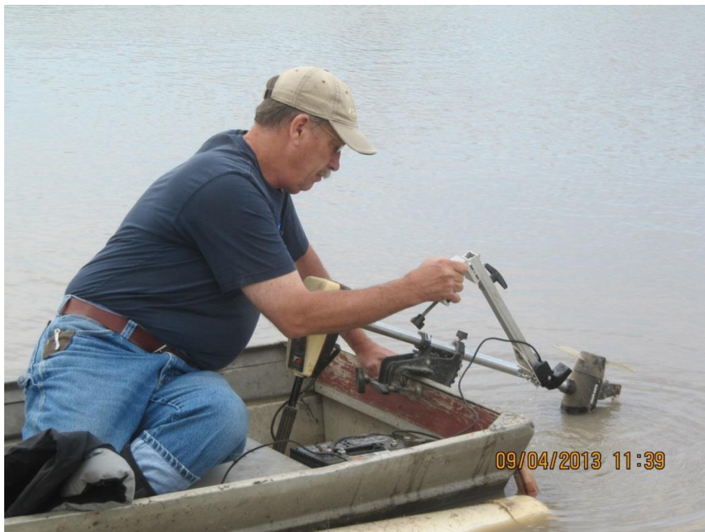
Figure 10 Close-up of transducer mounted to transom mount, about to be lowered into water and then depth adjusted.
