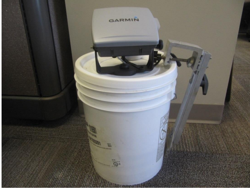
Figure 1 5-gallon bucket lid-mounted Garmin GSPmap 536s sounder/depth finder system. Transom mount (at right) resting on bucket lid.
