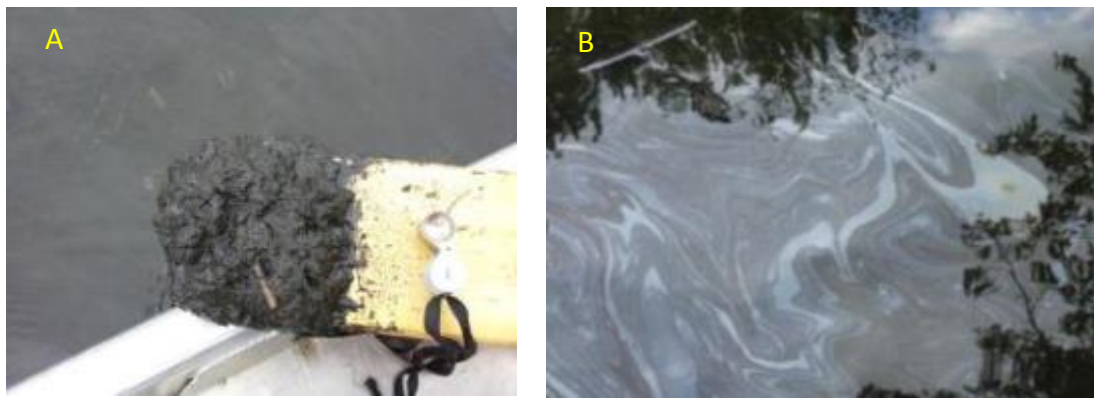
Figure 2 Photos from the Kalamazoo River: (A) Oiled soft sediment in the vicinity of the Ceresco impoundment in 2012 and (B) typical oil sheen and globes on the water surface near soft sediment deposits in the Battle Creek Millponds in 2013.
