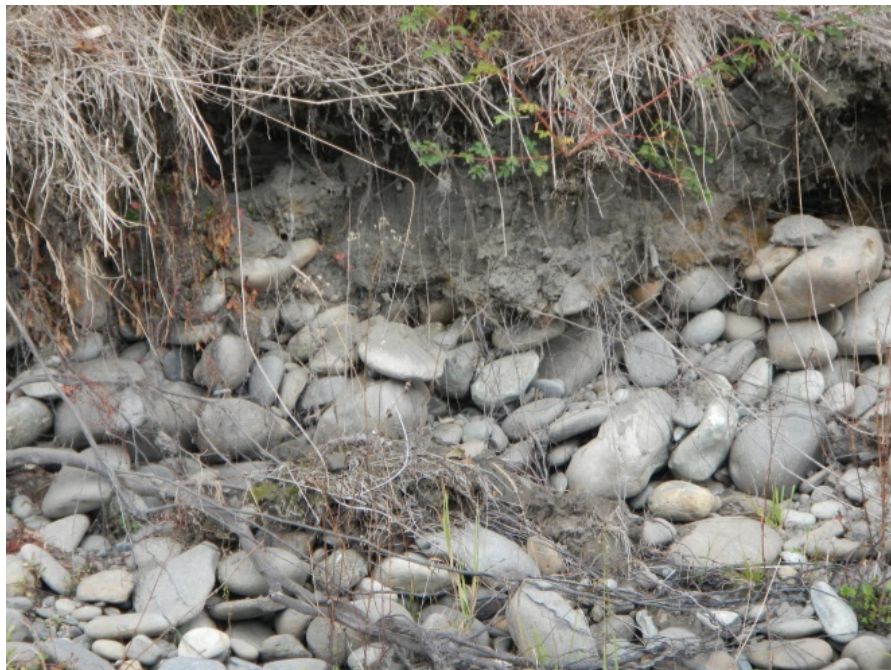
Figure 2 Close up of the streambank of the remnant floodplain shown in the right part of Figure 1. This figure shows a cantilever overhang that is sloughing as described by Reckendorf (2009 and 2010).
