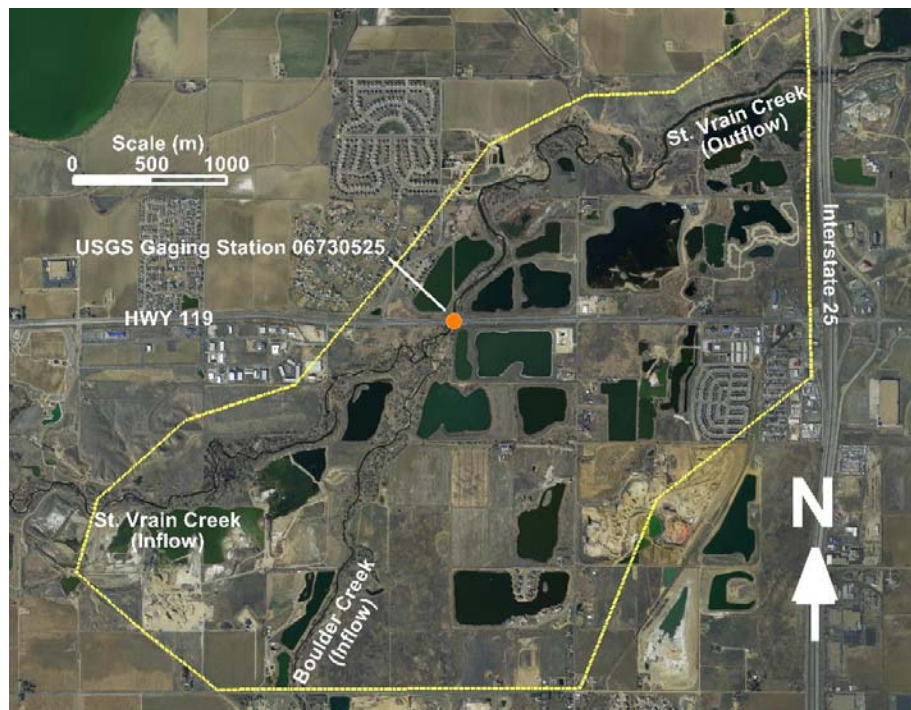
Figure 3 Aerial photograph of the modeled region. The limits of the computational grid are given by the yellow polygon shown. Note the inflowing tributaries at the south (Boulder Creek) and southwest (St. Vrain Creek) and the outflow boundary at the northeast (St. Vrain Creek). The circle marks the location of the USGS Gaging Station. (Photo source: USDA Geospatial Data Gateway.)
