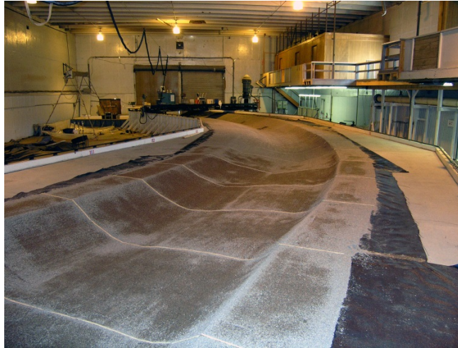
Figure 3 Completed native-topography downstream bed surface
