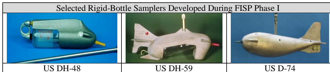
Figure 1 Examples of suspended-sediment samplers developed during Phase I of FISP.
