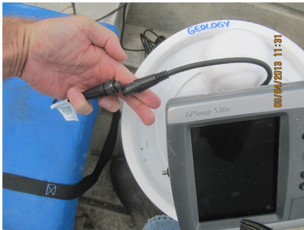
Figure 12 Cable connection from depth finder (right) to transducer cable (left).
