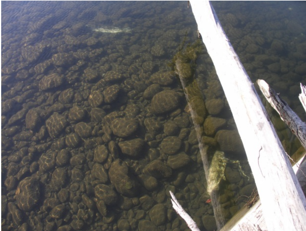
Figure 4 Coarse bed material next to an ELJ prior to dam breach.
