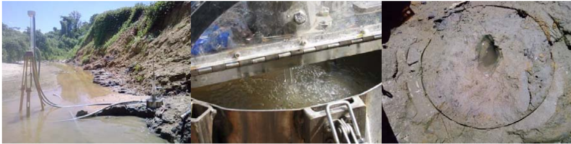
Figure 4. View of the a) jet test device setup, b) jet of water applied on the streambank material, and c) scour generated on the streambank material after a test
