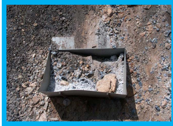
Figure 2 Hillslope erosion sediment collector trap.
