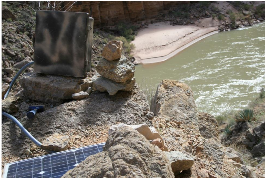
Figure 1 Typical setup of a remote camera system, at river mile (RM) 145.9, Grand Canyon. Visible is the waterproof box containing camera and electronics, and the 20W solar panel.
