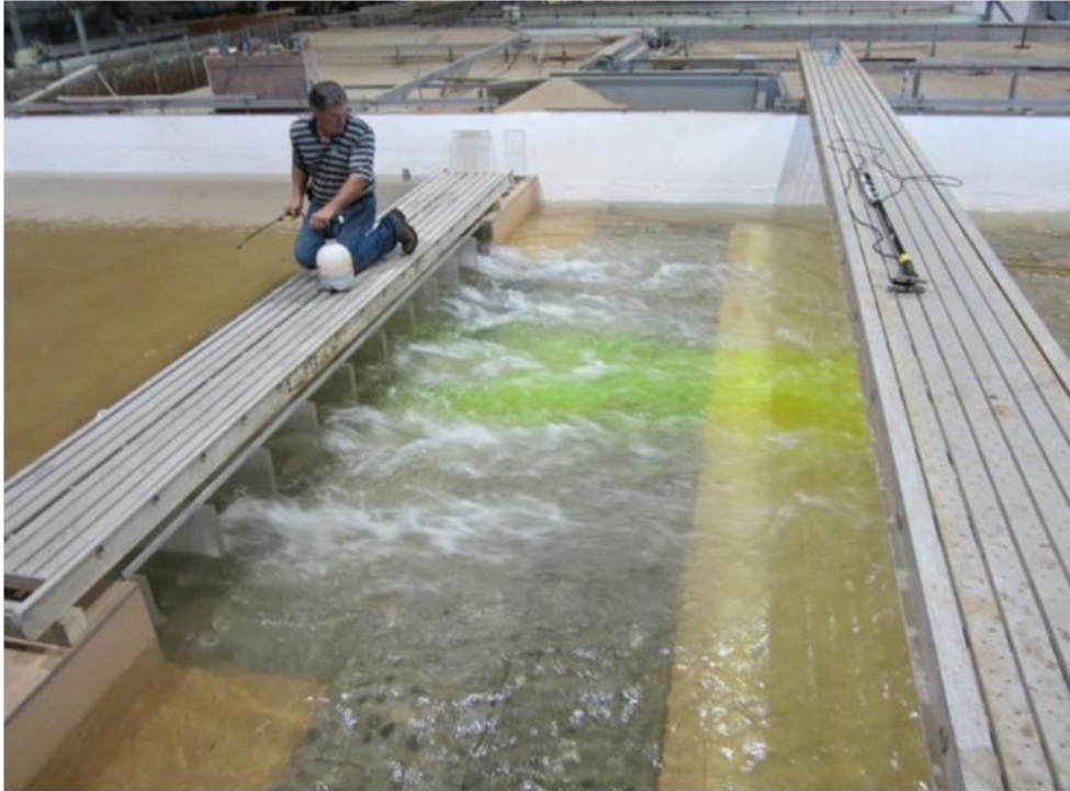
Figure 13 MCS Physical Model with Plunge Pool Experiment
