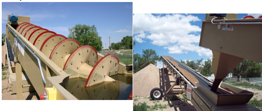
Figure 4 Archimedes screw separator (left) and stacker (right).
