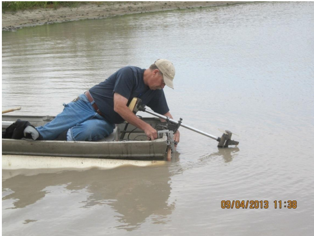
Figure 11 Transom mount screw clamp being tightened and transducer adjusted to proper reading depth. The transducer depth is then measured from the water surface (and recorded as a correction factor).
