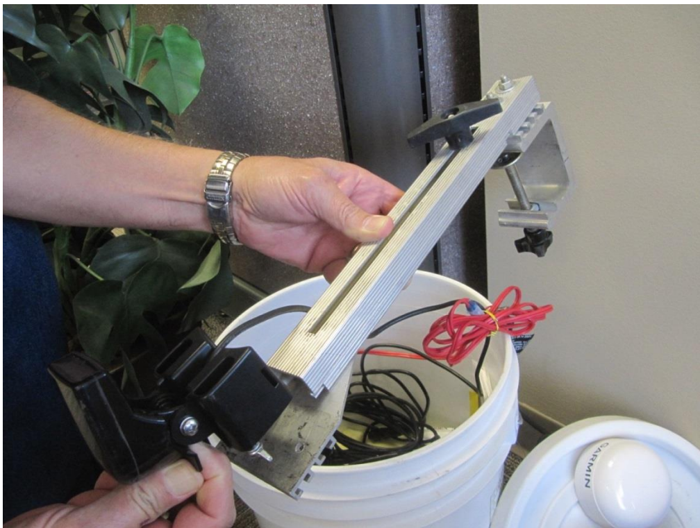
Figure 4 Transducer (lower left) shown where it is to be bolted to the bottom of the transom mount and depth adjusted on site. External GPS antennae shown mounted to bucket lid.
