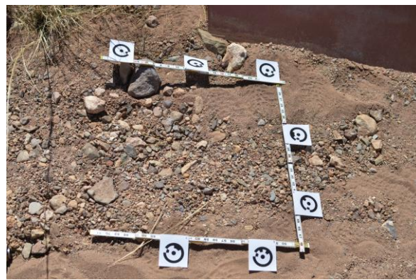
Figure 1 Left: Particle size distribution (mm) from three samples taken along the Lucky Hills watershed main channel. Large fractions of sandy loam and coarse angular material resulted in a bimodal size distribution. Right: Photo of typical coarse sediment deposits along the ephemeral channel.
