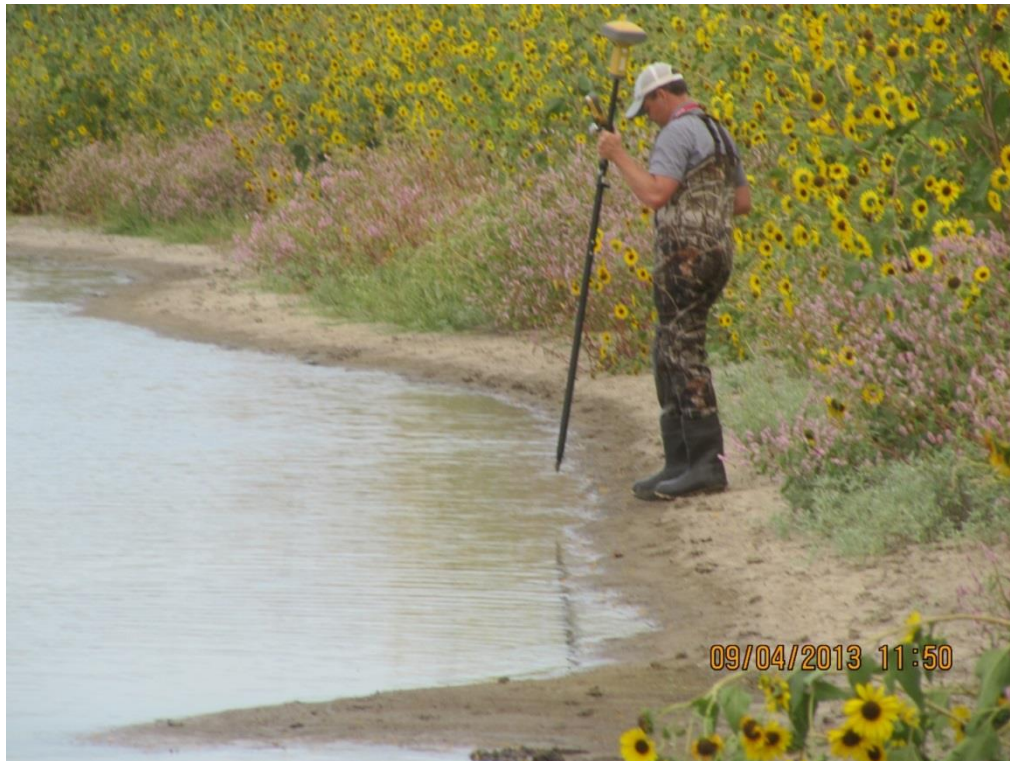
Figure 6 Shoreline survey using survey grade GPS system provides a zero depth for bathymetric survey.
