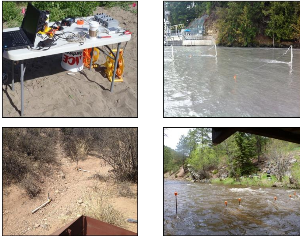
Figure 1 Top Left: Photograph of the first iteration of the passive acoustic bed load monitoring system, deployed at Douglas City on the Trinity River, CA. Top Right: Installation of three hydrophones at the Elwha River, WA. Bottom Left: Installation of two hydrophones at the Lucky Hills subwatershed near Tombstone, AZ. Bottom Right: Installation at the Bear Creek, near Denver, CO
