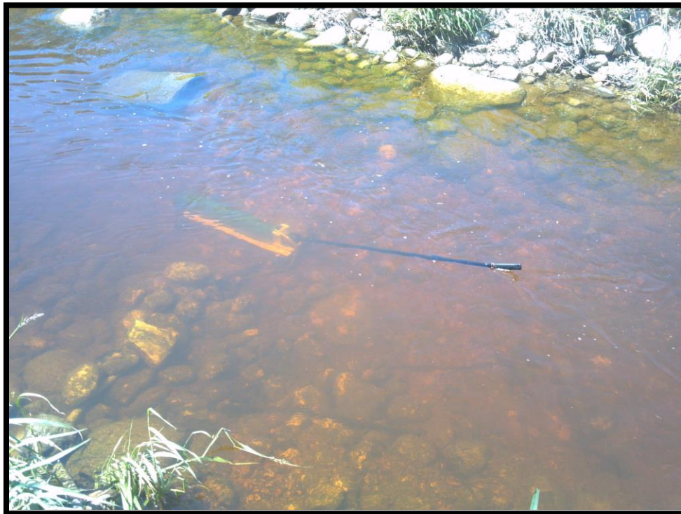
Figure 2 Image of the DISA in an open channel setting. The body is anchored to the streambed with the sample arm oriented in the downstream direction. Photo by USGS.
